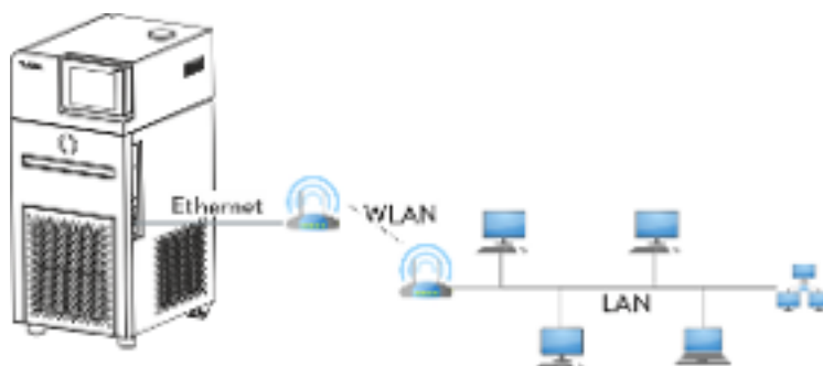
Fig. 16: Connected via LAN and WLAN
