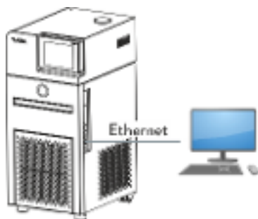
Fig. 14: Connected via Ethernet cable
