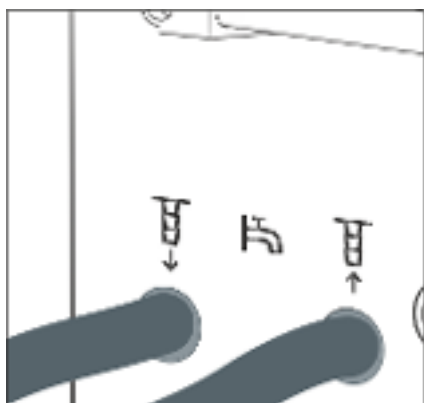
Fig. 23: Cooling water input and output
